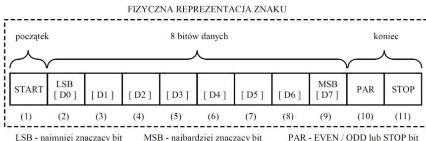
Figure 8. Character format in the MODBUS RTU standard used in the transducer.
