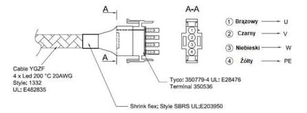
Due to the length of the motor cables, extension cables are additionally provided to connect the motor to the controller. The extender is equipped with 4-pin connecting sleeves that fit the motor terminals.
