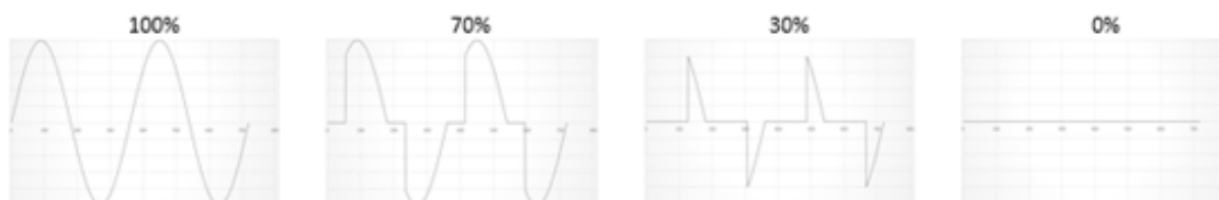
Figure 3 - modulating the supply voltage depending on the demand for heating power
