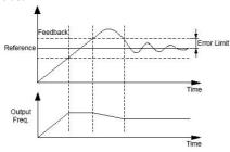
Fig. F8-3 Error Limit Schematic Diagram
