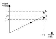
Fig. F5-4 Voltage Control Mode 0
