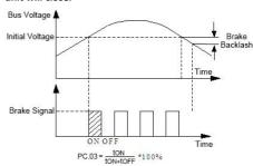
Fig. FC-1 Dynamic Braking
