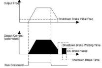
Fig. F1-4 Stop DC Braking
