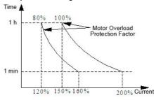
Fig. FA-2 Motor Overload Protection Factor Setting
