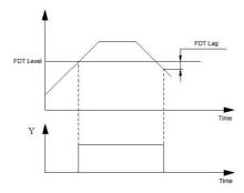
Fig.F7-8 Frequency Level Detecting
