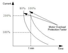
Fig.FA-1 Motor Overload Protection Factor
