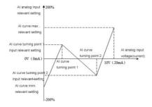
Figure F6-2 Almulti point curve diagram
