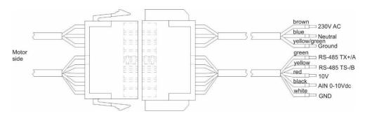
Fig.16b. EC motor cable description
