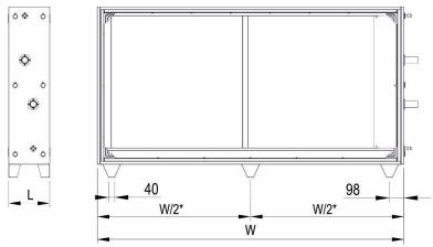
Fig.5. Supports of the short (L≤630mm) sections
