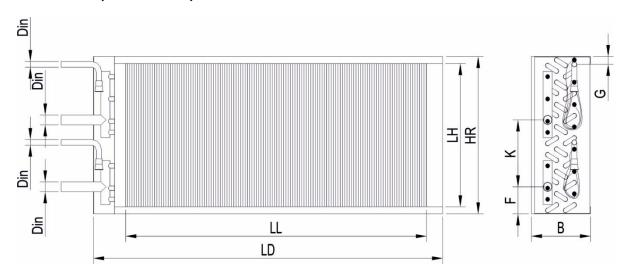
Fig. 35 Two-circuit (Two-section) DX coil
