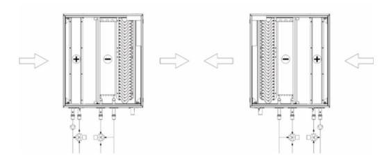
Fig.10. Examples of feeding water exchangers
