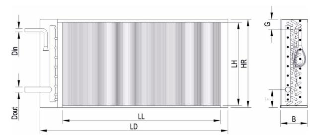
Fig. 24 One-circuit (One-section) DX coil
