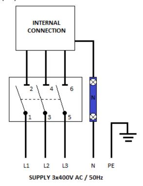
Power supply connection for circulation pump for the water heater, connector 1, N, PE at the main disconnector.
