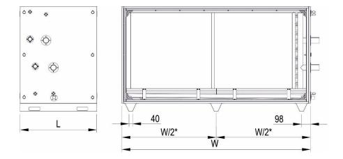
Fig.6. Base frame profiles of VVS 21-150 AHUs
