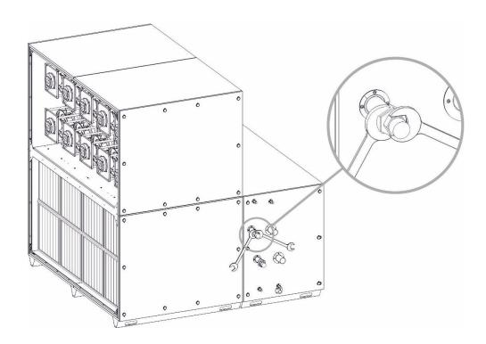
Fig.9. Securing the screwed connections of the exchanger
