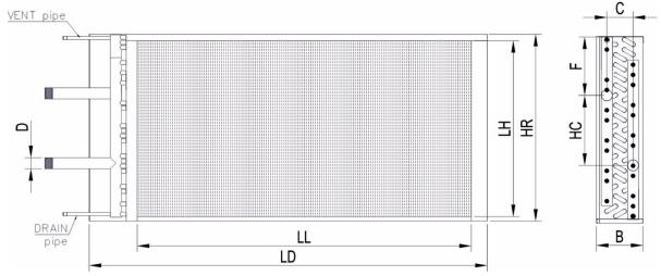
Fig. 13 Dimensions of hydronic coil exchangers
