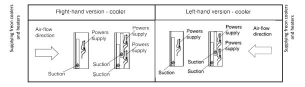
Fig. 11 Supplying freon coolers and heaters
