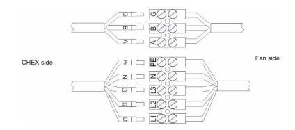
Fig.16a. Fan electrical terminals
