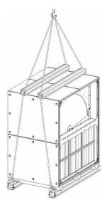
Fig. 4b. Transport with the use of a crane
