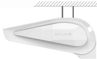
SCHEMA DI MONTAGGIO CON BARRE FILETTATE INSERITE NEGLI INSERTI
