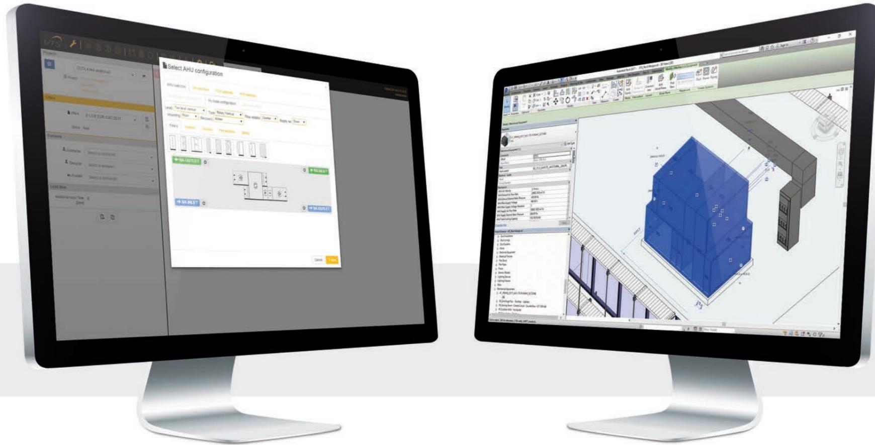
The release of so called families for the Autodesk Revit® environment by VTS makes it easier to design agencies to model the building installations on the basis of using the same platform. At present the on-line generator is a unique solution in BIM environment. It enables the generation of a VENTUS air-handling unit model practically in no time in any configuration and with any parameters.
