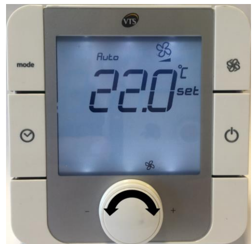
Figure 33 - HMI Basic. Temperature set-point
