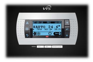
Operation is done via 6 buttons on both sides of the screen.
