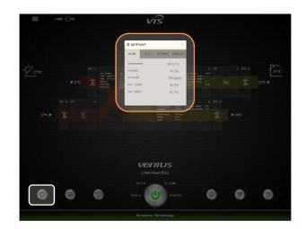
Each operating mode has all parameters set separately: Temperature / humidity / air quality / fan supply and return control
